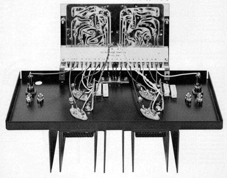
This completes the soldering to holes on the foil side of PC-36, and to most of the connections on the back panel. Now you should check all your connections. See that no solder blobs or excess wire connects other than the intended terminal. Cut off any excess wire on the other side of a connection with your side cutters. Turn the assembly over and cut off any excess wire (more than ½6"—.2 cm) from the soldered holes on the board.
