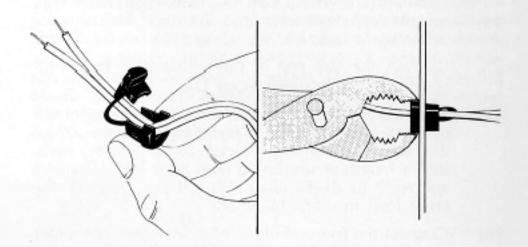
25( )Select the conductor with 1" (2.5 cm) of insulation removed. Feed it through power switch lug #1 to power switch lug #2. Solder both lugs.
