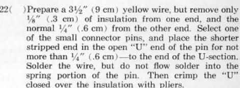
spring portion of the pin. Then crimp the "U" closed over the insulation with pliers.
